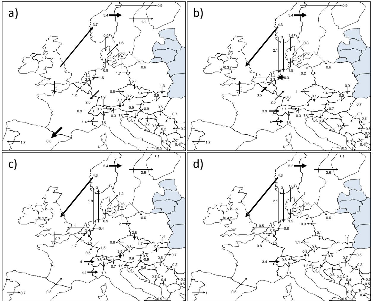
Figure 8: Cross-border flows in GW on a typical summer weekend day with a) high and b) low RES infeeds and low load at noon, as well as a typical winter working day with c) high and d) low RES infeeds and high load in the evening (7 p.m.)
